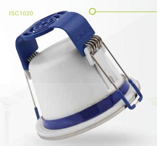
The Insulation Support Clip has been developed to allow installers to lay thermal insulation directly over the top of the Inceptor® Pico FG. It creates a 20mm air-space above the driver which allows air to circulate and cool. This allows the driver to dissipate heat more effectively and in-turn allows the luminaire to run cooler.
